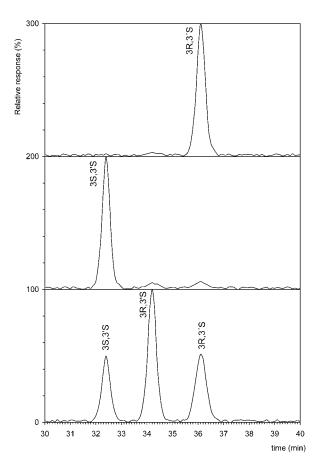
Figure 1 HPLC comparison of astaxanthin isomers found in alga, yeast and synthetic astaxanthin. Column CHIRALCEL® OD-RH, 150 x 4,6 mm, 5 μm was used with mobile phase acetonitrile/phosphoric acid (3.5 mM) at a flow rate of 0.5 ml/min under isocratic conditions and a temperature of 25 °C. Identification of astaxanthin peaks was achieved by using the wavelength of 470 nm (Rezanka et al., 2013).
